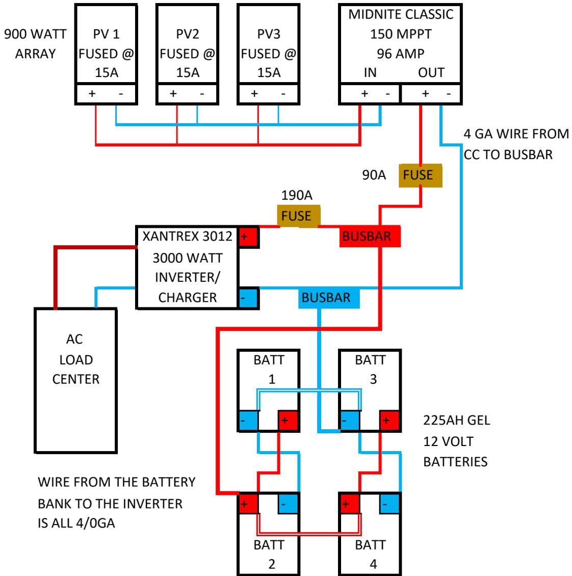
Battery bank is wired in parallel using Method 4 on the Smart Gauge Website
