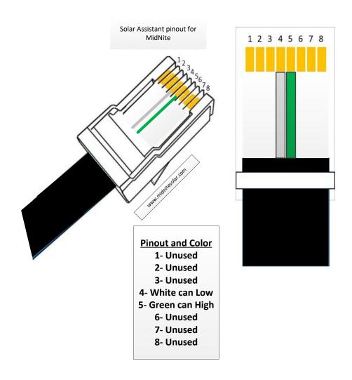
To connect the Solar Assitant to the Midnite Rosie / MNGP2 / Hawke's Bay or Barcelona simply unplug one of the blue terminator plugs on one end of the canbus in the system and plug in the solar assistant cable.
