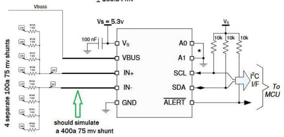
2) My simulations show that the resistor divider network acts like a 400a 75mv shunt. Are these calculations correct?
